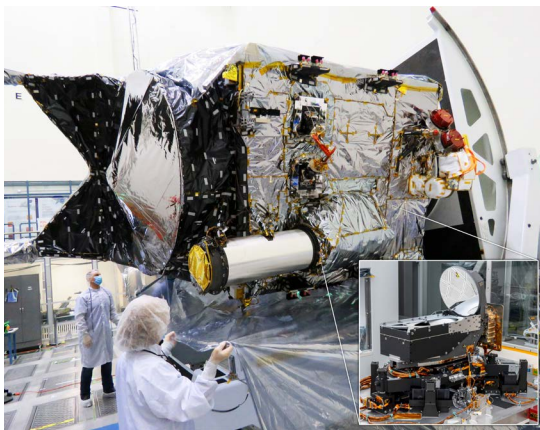
DSOC's flight transceiver can be identified by its large tube-like sunshade on the Psyche spacecraft, as seen here inside a clean room at JPL. Inset: An earlier photo shows the transceiver assembly before it was integrated with the spacecraft. Credit: NASA/JPL-Caltech
